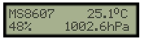
Sensor measurements are refreshed every 500 milliseconds.
