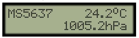
Sensor measurements are refreshed every 500 milliseconds.
