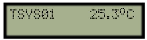
Sensor measurements are refreshed every 500 milliseconds.
