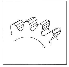
A pole wheel on the target shaft is required when using contactless sensors to generate a signal. Often an existing gear wheel can be used but where none is present a special gear, slotted or holed disk would be added.
