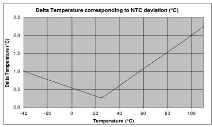
0.1°C tolerance on Resistance Measurement
