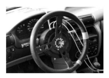
Mounting principle of transducer on steering column - no disassembly of column is required.
