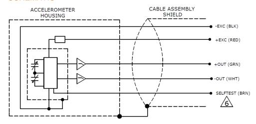
BIT: CONNECT TO CIRCUIT GROUND TO PERFORM SELFTEST WHICH PRODUCES A 24Hz, 1g PEAK-TO-PEAK AMPLITUDE, SQUARE WAVE OUTPUT SIGNAL BY MECHANICALLY ACTUATING SENSOR ELEMENT. THE SELF-TEST OUTPUT SIGNAL IS IN ADDITION TO ANY INERTIAL ACCELERATION ACTING ON THE DEVICE DURING SELF-TEST. A ZERO-G ORIENTATION PROVIDES A ±0.5g SELF-TEST OUTPUT SWING AROUND ZERO-G BIAS. AN AC VOLTMETER DISPLAYS A 0.5g-rms EQUIVALENT OUTPUT SHIFT. A SINGLE-ENDED HOOKUP REDUCES THE SELF-TEST OUTPUT BY HALF.
